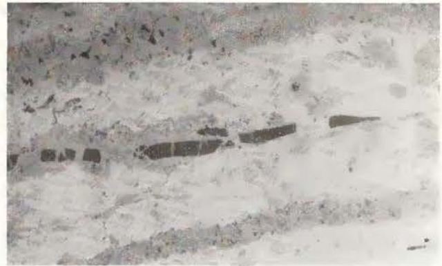
Fig. 18. Polished section of iron fragment JAK 7, showing fractured glassy inclusions (450 X).
