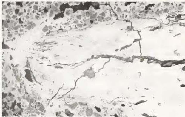
Fig. 7. Polished longitudinal section through the tip of iron bar JAK 3, showing the preservation of the original outline (36 X).
