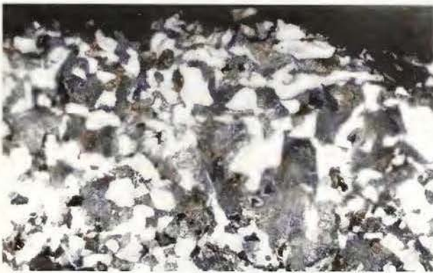
Fig. 17. Etched section of metal in JAK 7, showing white ferrite and dark coarse pearlite (280 X).
