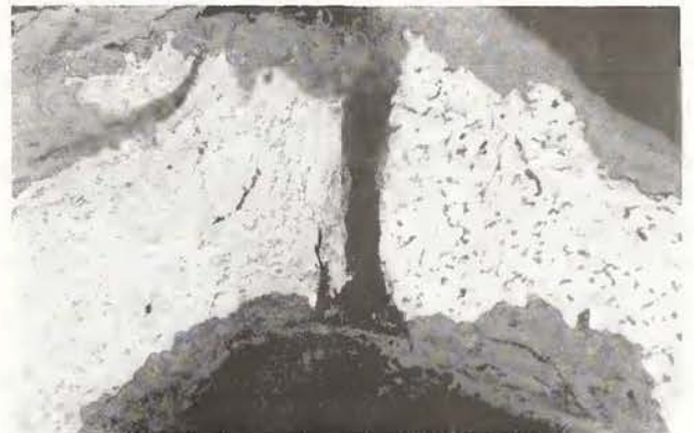
Fig. 12 Etched section of iron bead JAK 5, showing grain deformation at the join (56 X).
