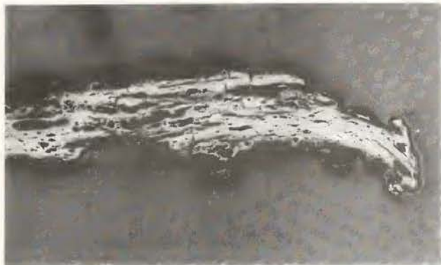
Fig. 25. Polished section of corroded iron strip JAK 11 (7 X).
