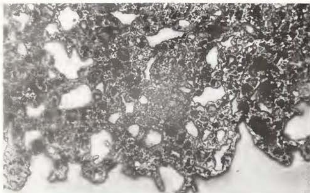
Fig. 13. Polished section of glassy nodule JAK 6B, showing irregular porosity (7 X).
