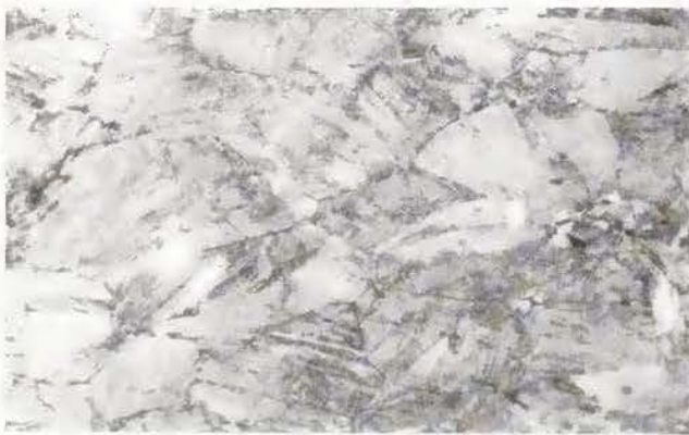
Fig. 6. Etched longitudinal section of brass cap JAK 2, showing slip bands in intensely deformed grains (140 X).
