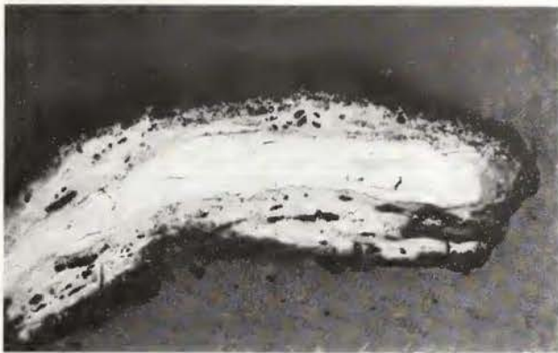
Fig. 16. Polished transverse section of iron fragment JAK 7, showing curved cross-section (7 X).
