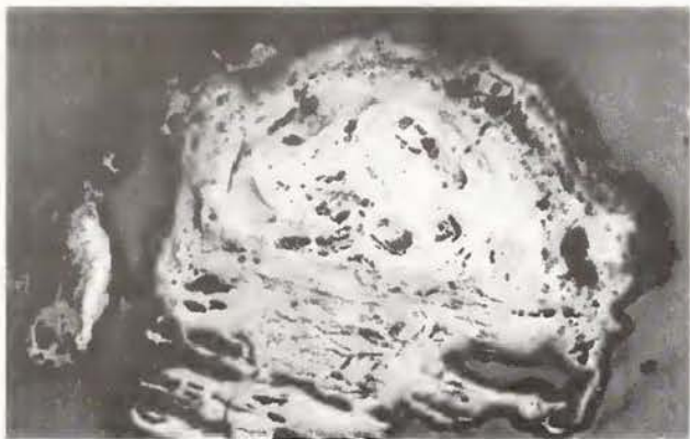
Fig. 5. Polished transverse section of iron rod JAK 1, showing the severe corrosion of the iron bar (9 X).
