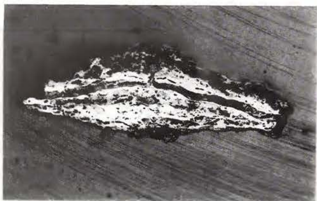
Fig. 22. Polished section of corroded iron strip JAK 9 (7 X).
